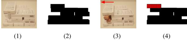
Fig. 12: Stability analysis for package palletization. Black: stable bricks. Red: collapsing bricks.
